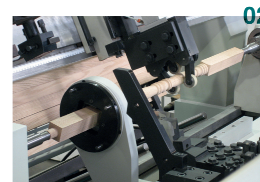
Optional equipment: Pneumatic steady with three rollers to avoid the vibration when turning thin and long pieces.
