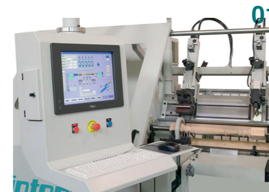
Standard machine: 2 CNC copiers, hopper feed loader and 2 automatic back knife units.
