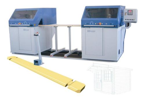
Double end Log cabin milling machine Blockhausfräse BL Twin for serial production of components for garden log Cabins.
