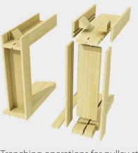
Trenching operations for pulley stiles and cutting of lining beads
