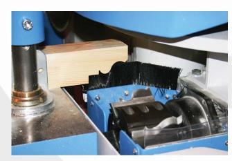
Horizontal milling unit for heritage sash horn detail or trenching of sash box
