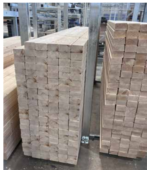
▲ Storing the studs in racks
